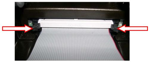
Figure 3-3 Release the Ribbon Cable
