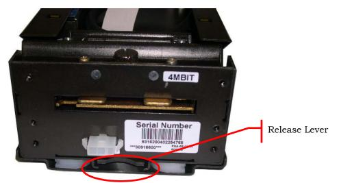
Figure 3-4 Press the Release Lever
