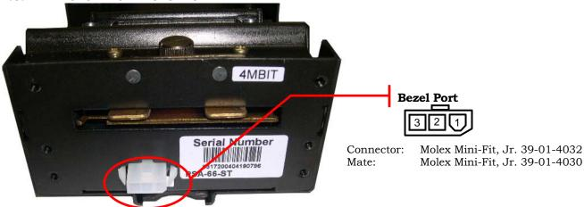
Figure 4-3 RS232 Front Bezel Port
