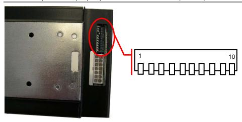
Figure 4-5 RS232 Dip Switches
