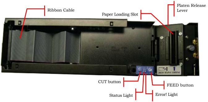
Figure 2-1 Operator Indicators and Controls
