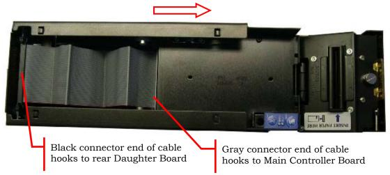
Figure 3-5 Remove the Printer
