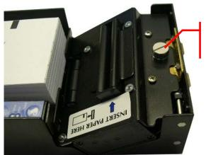
Mechanism Fastening Screw
