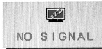
Turn off the LCD monitor and reconnect signal cable, and then turn the computer and LCD monitor on.
