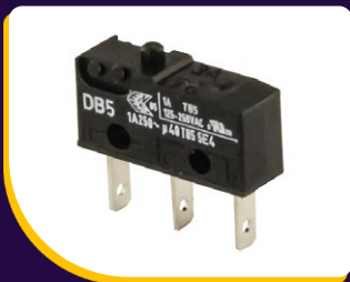
Cherry Sub-Miniature Switch 1 Amp 125/ 250V .110" Terminal DB5G-B1AA 70 Gram
