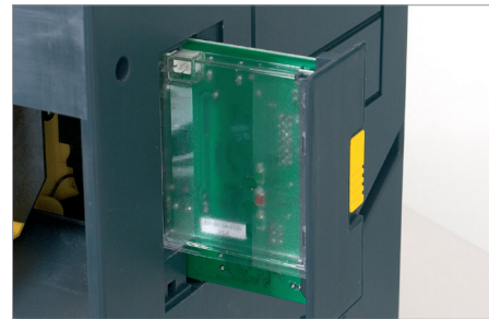
Board easily extractible from the outside
