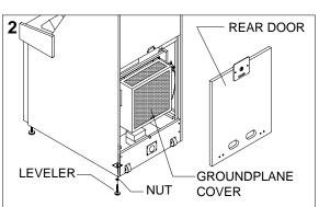
Unlock, remove and set aside rear door. Remove groundplane cover. Ensure major assemblies and cable connectors are mounted securely and fan airflow is unobstructed. Do not force connectors. Tilt cabinet to locate four threaded holes on bottom. Install leveler and nut into each hole, but do not tighten yet.
