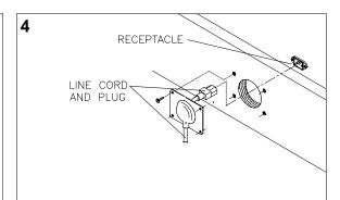
Remove and save four screws from line cord cover plate at cabinet rear. Remove cover plate. Match holes on IEC plug with prongs in receptacle and push firmly to seat line cord. Hold cord flat against cabinet and reinstall cover plate (indentation points down so cord exits toward bottom of cabinet).
