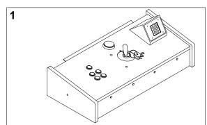
Remove items from shipping container. Inspect cabinet exterior for damage.
