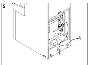
Uncoil telephone cable inside cabinet. Run cable through notch in cabinet rear and plug into working telephone jack. Replace groundplane cover, taking care not to pinch wires or cables. Replace and lock rear door.
