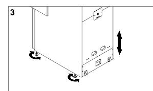
Stand cabinet upright and make certain it is in a stable position. Move game to its intended location and level the cabinet. Game is intended for use only in a fixed position. Ensure that final adjustment raises game so swivel caster wheels do not touch the floor. Distribute weight equally on each corner and tighten leveler nuts.
