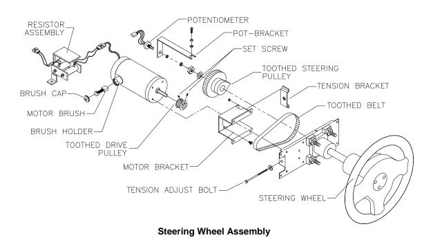
Inspect the motor, pulleys, and belt. If the belt is broken or shows signs of wear, replace it. Locate the two nuts on each side of the motor mounting bracket. Loosen all four bracket nuts. Rotate the tension adjustment bolt as necessary. Tighten this bolt until the belt is taut. Then restore correct tension by loosening the bolt one full turn. Tighten the motor bracket nuts.
