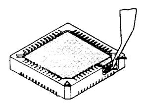
**9)** Pull the tool back away from the socket using slight downward pressure until the corner of the chip lifts away from the socket.
