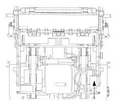
**2)** Remove the 2 screws holding the cable clamp in place. Then disconnect the Led harness, Optics housing, and the Stacker housing.
