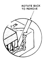
**10)** Repeat on the opposite extraction slot and lift chip out of the socket.
