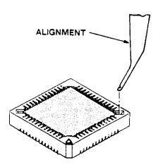
**8)** Lower the extraction tool into the extraction slot until it bottoms out.
