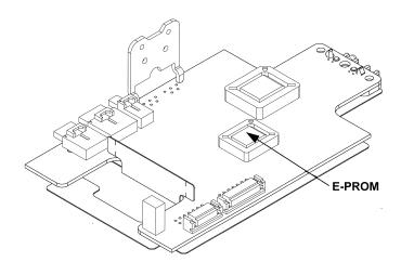
**6)** Remove the chip from it's socket. Use an Amp extraction tool for plastic leaded chip carriers (E-Prom Replacement Kit Part Number 210826001) or equivalent tool. Locate the extraction slots.
