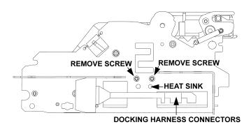
**4)** Remove the two screws connected to the Bob Sensor on the control board. Then slide the control board out of the RTU.
