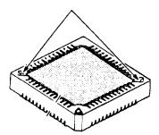
**7)** Insert the extraction tool into the socket so that the front angle of the tool is perpendicular to the socket.
