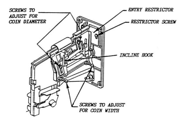
MECH MUST BE MOUNTED UPRIGHT AND VERTICAL WHILE ADJUSTMENT IS BEING MADE.
