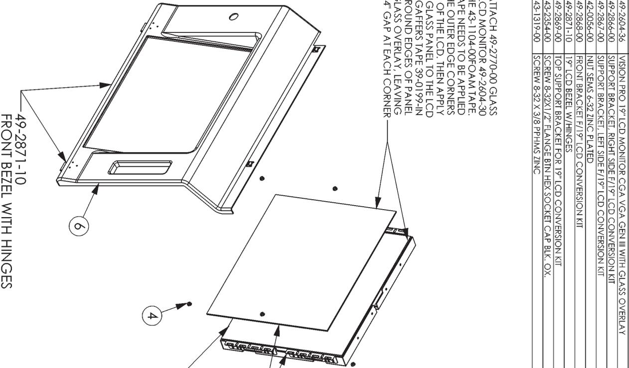
INSTALL TOP BRACKET ON SIDE BRACKETS USING 8-32X 3/8 SCREWS (43-1319-00) DON'T SCREW 8-32 X 1/2" FLANGE SCREWS TO THE CABINET UNTIL 19" LCD HAS BEEN INSTALLED FIRST. THEN TIGHT FLANGE SCREWS FROM TOP OF CABINET
