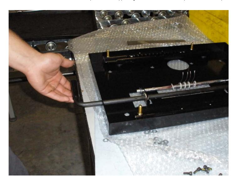
8: Apply a thin coat of grease to the edge of the Spring Tensioner as shown below.
