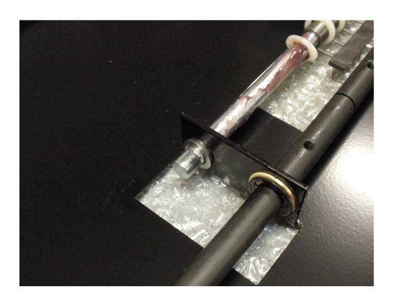
6: Secure Shaft Spring Rider with external retaining ring heavy duty at both ends of the shaft spring rider in slots provided for this purpose.
