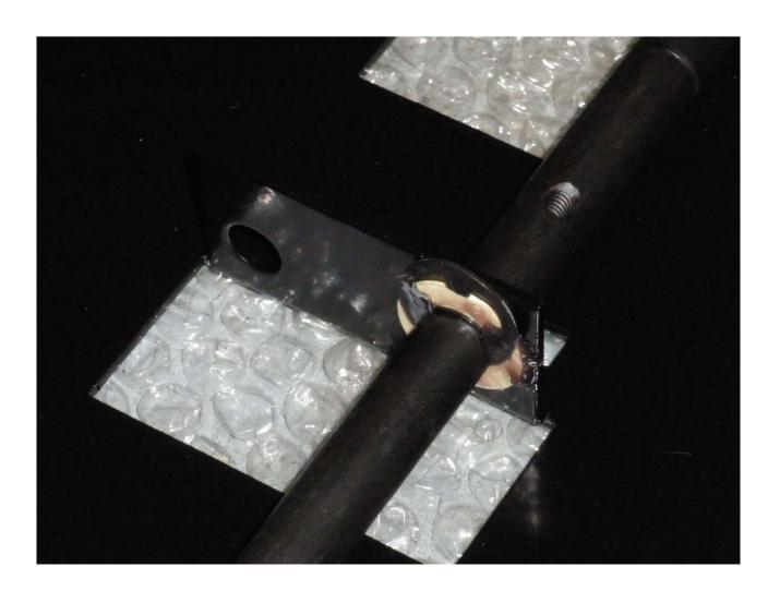
Slide Shaft Spring Rider with springs and plastic spacers (illustrated in step 1 above) into hole adjacent to hole where lever arm has just been re-installed in step 4 above. Install into hole closest to back of seat slide base first 5: as shown below.
