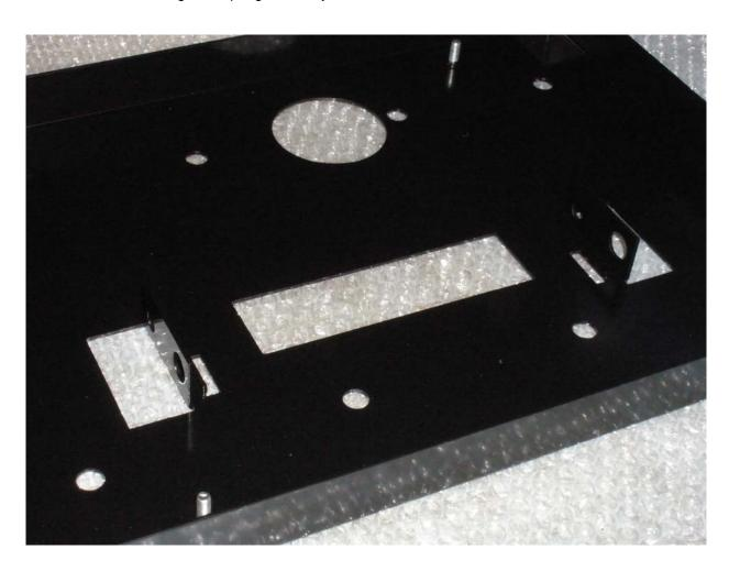
3: Install Plastic Bushings into holes where Lever arm will pass through on Seat Slide Base and apply light coat of grease to inside of bushings.
