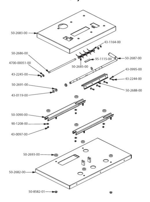
1: Apply light coat of grease to shaft spring rider.
