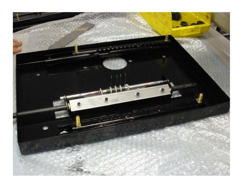
10: When assembled correctly the Springs, Spring Clip, Plastic Spacers, and Shaft Spring Rider Assembly should look as it does below.
