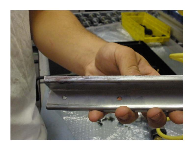
9: Attach the Spring tensioner to the lever arm using part numbers 43-0995-00 # 10 SAE Flat Washer 43-2244-00 10-24 X ½" socket head cap screw (4 places) as shown below. When installing this piece make certain that the Spring Clip is under the inner surface of the spring tensioner. Tighten these screws securely. See four photos below.
