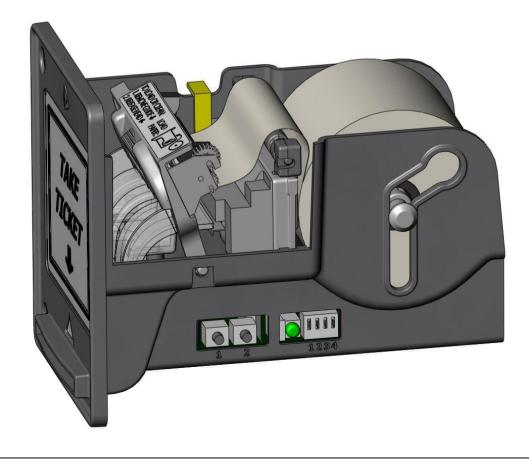
**Second Method:** (See Figure 2) cut or rip the end of the paper roll so that a nice flat edge is present. Hold this edge into the head mechanism. In a few seconds, the head will slowly pull in the paper. It will then speed up and then feet out about 12 inches of paper.
