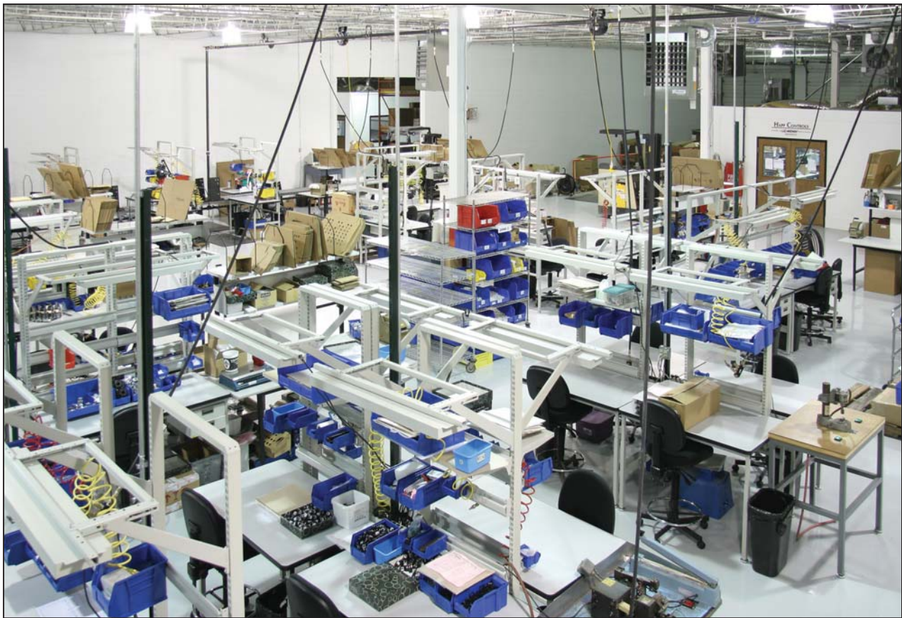
The Happ factory floor was converted from a traditional production model to a cellular one.
