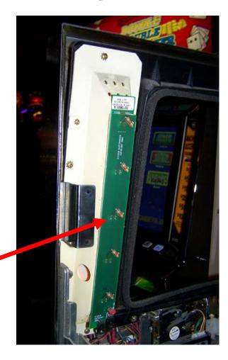
Note: on machines with LCD conversions, you must install the pcb with connector up and use optional K902-106E extension adapter. Direct short circuit will occur if you install with connector down position!!
