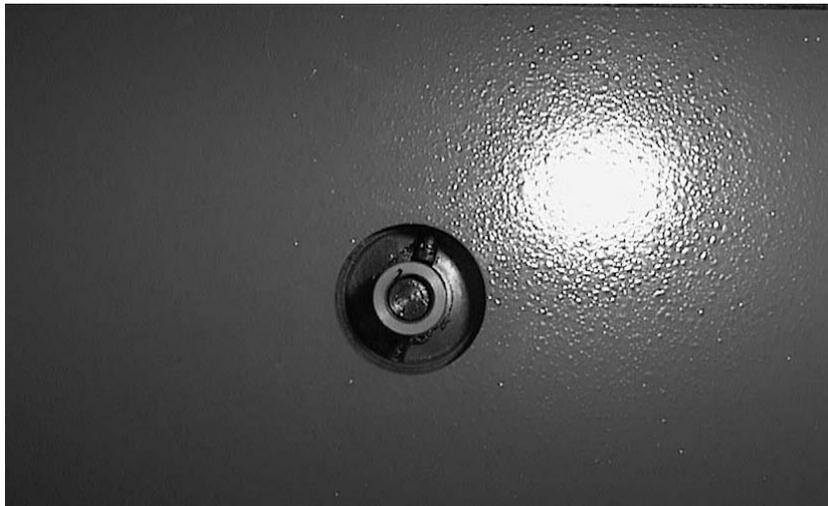
**Crank Handle shaft located on right side of Coin Counter**
