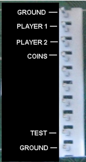
Figure 8. 10 Pin Molex connector pin layout
