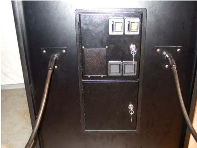
**Figure 3. Gun Mounting Plates Attached**
