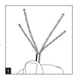
Separate pairs and lay out per the T568A or T568B specification required for your application. Use the convenient color chart on the EZ-SnapJack wire guide to assist you.
