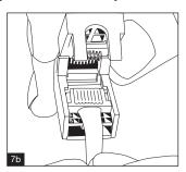
Push down on the **EZ-SnapJack until it** snaps completely shut.
