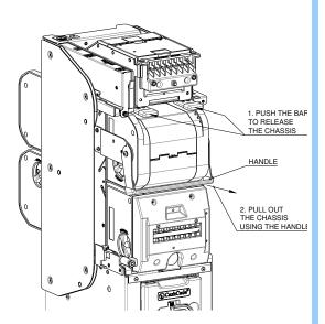
Caution! The chassis may be heavy to handle! Support the module beneath the chassis with one hand.
