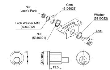
How to install the lock on the dispenser module
