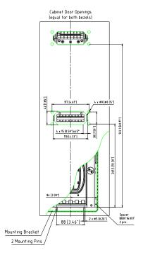
Recommended door openings for bezels installation
