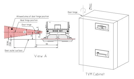
**Door Hinge – Bezel Installation Alignment**
