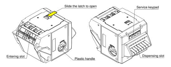
A standard 3/4" tubular lock can be installed in the dispensing cassette, which will allow the chassis to be secured to the recycling cassette module, and the dispensing cassette inside the housing. There is a placement for a lock under the dispensing slot.
