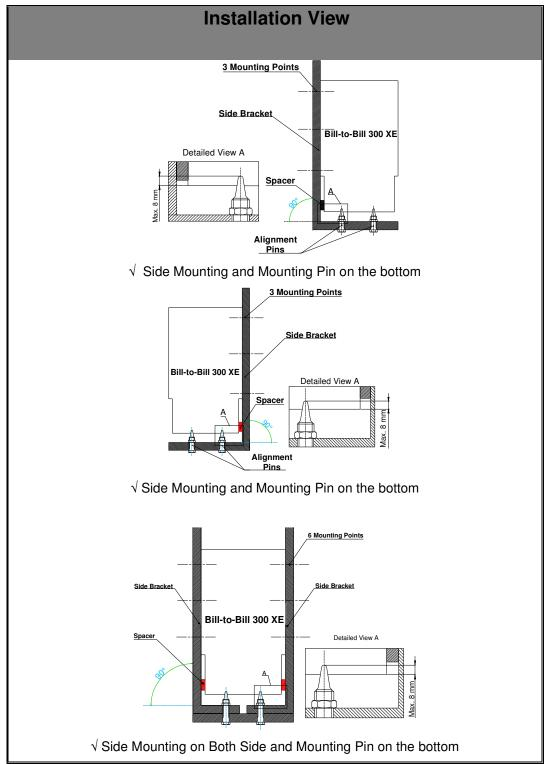
**Recommended Mechanical Installation Method**
