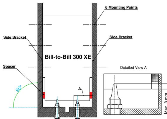
√ Side Mounting on Both Side and Mounting Pin on the bottom
