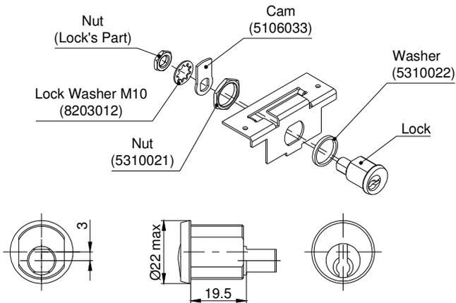
How to install the lock on the dispenser module
