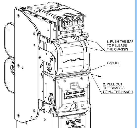
**⚠ Caution! The chassis may be heavy to handle! Support the module beneath the chassis with one hand.**
