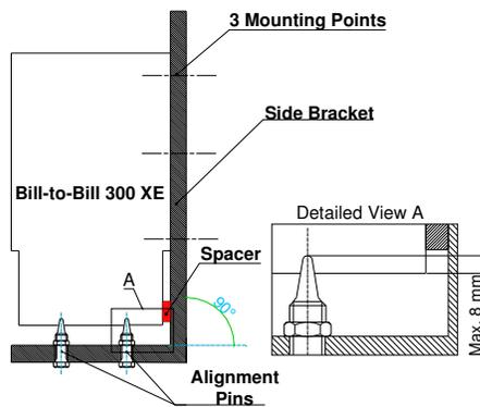
√ Side Mounting and Mounting Pin on the bottom
