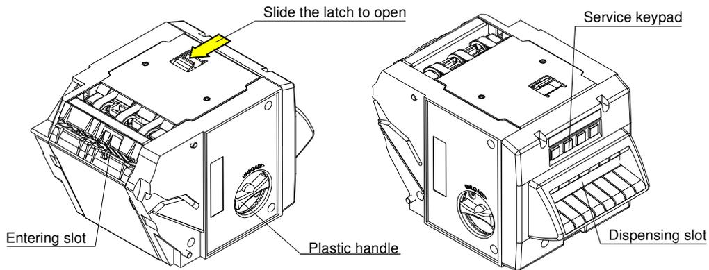
A standard 3/4" tubular lock can be installed in the dispensing cassette, which will allow the chassis to be secured to the recycling cassette module, and the dispensing cassette inside the housing. There is a placement for a lock under the dispensing slot.
