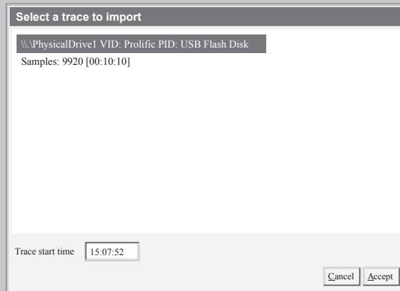
Figure 12 - SD card import list. This is useful to read an SD content without the SMA unit
